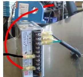
Above Mean Well power supply and Hall-effect current monitor
