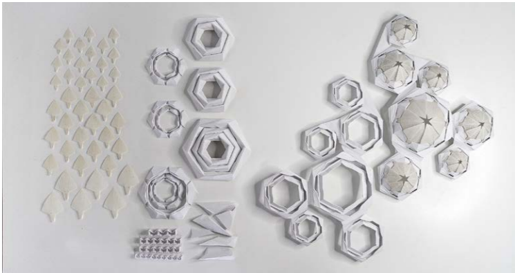
4. Multi-kinematic-state climate-responsive flap with doubly-curved deformation along primary axis (A) and secondary axis (B). Three states are presented: left, flat state after FFF under controlled environment; centre, convex double curvature under high R.H.%; right, concave double curvature under low R.H.%.
