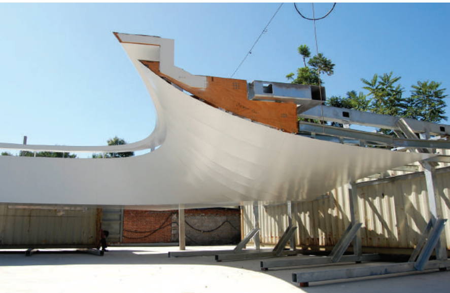
4: 3-mm aluminium material-test mock-up produced by Permasteelisa, October 2009. Several geometric conditions are explored as well as rationalisation testing. This mock-up was one of several material validation built to facilitate a material systems decision for executing the project.
