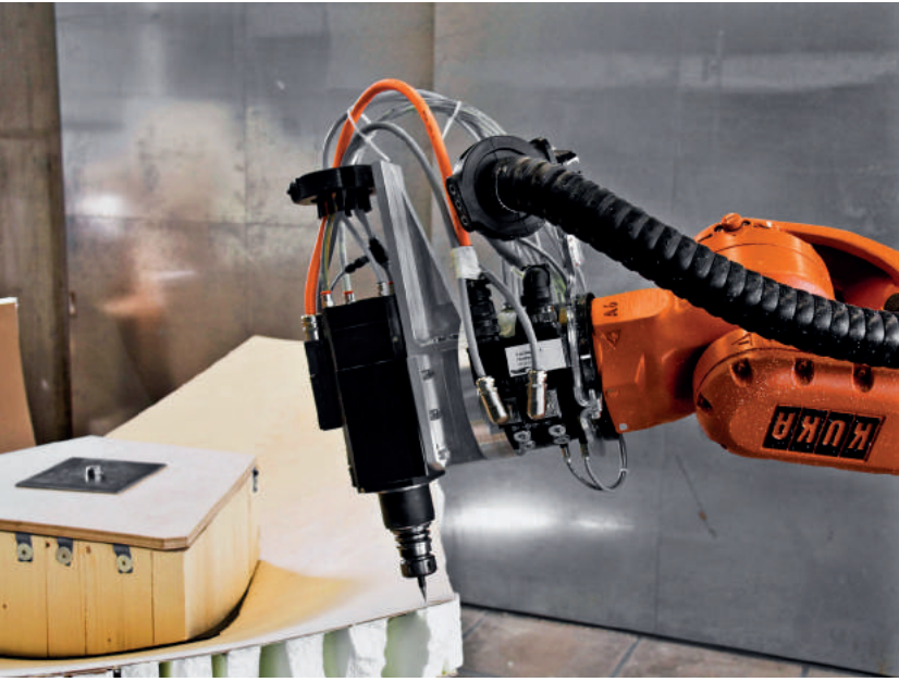
Fig. 7: Measuring the module's position before robotic cutting and milling.
