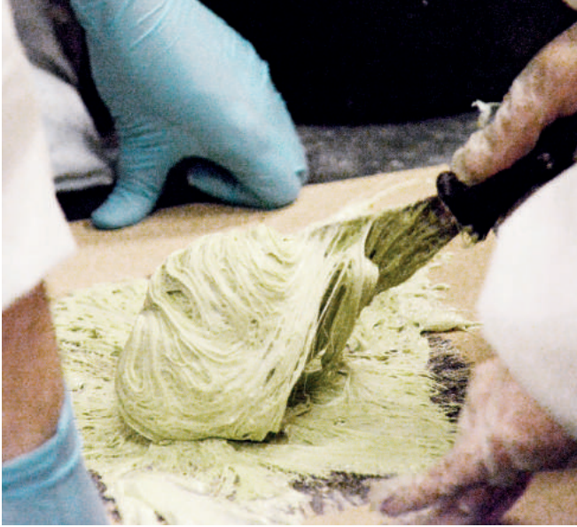
Fig. 6: Material mixture: depending on the desired result, the additive components include modelling plaster, water, hardener and colour pigments. Event: Robotic FOAMing, Smartgeometry 2013.
