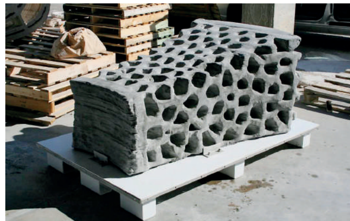
Figs. 10, 11: A large mock-up of the regolith shield was fabricated on the D-shape printer.
