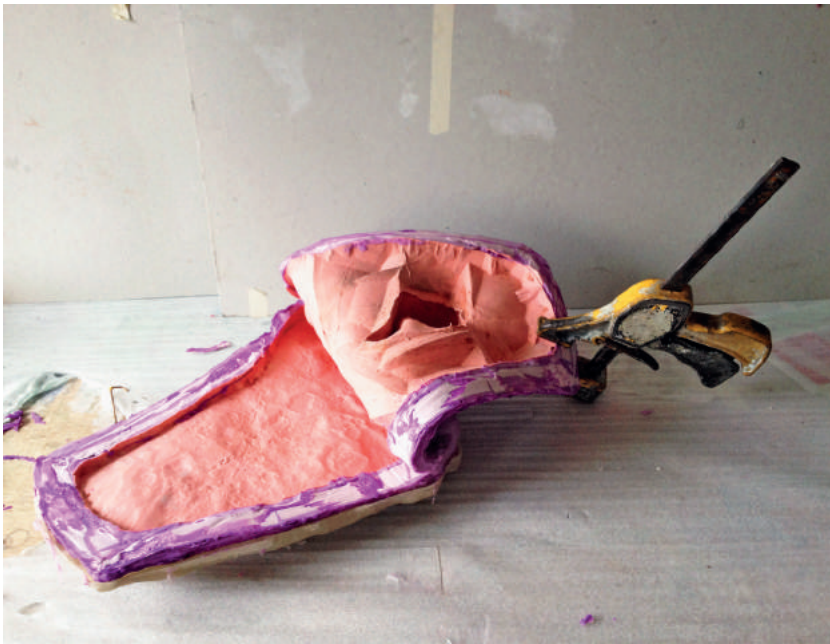
Fig. 11: One of the smallest one-part silicone moulds used to cast each Frozen Relic replica. The mould is seen here open with the split line lip for resealing exposed.
