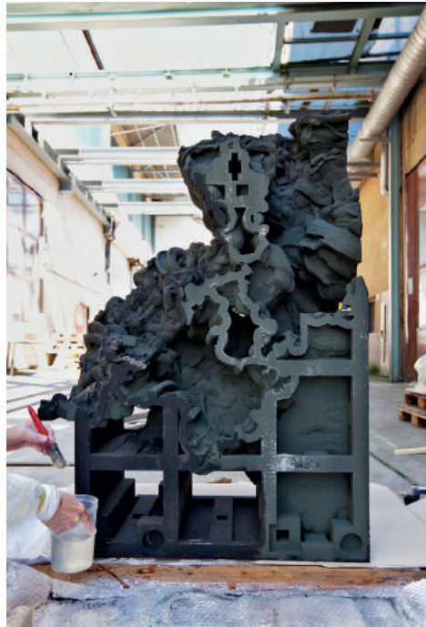
Fig. 5: Resin reinforcement of printed grotto element.
