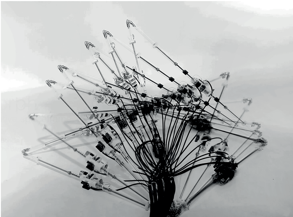
Fig. 12: Overlays for step cycle performed by the tetrahedral truss prototype.
