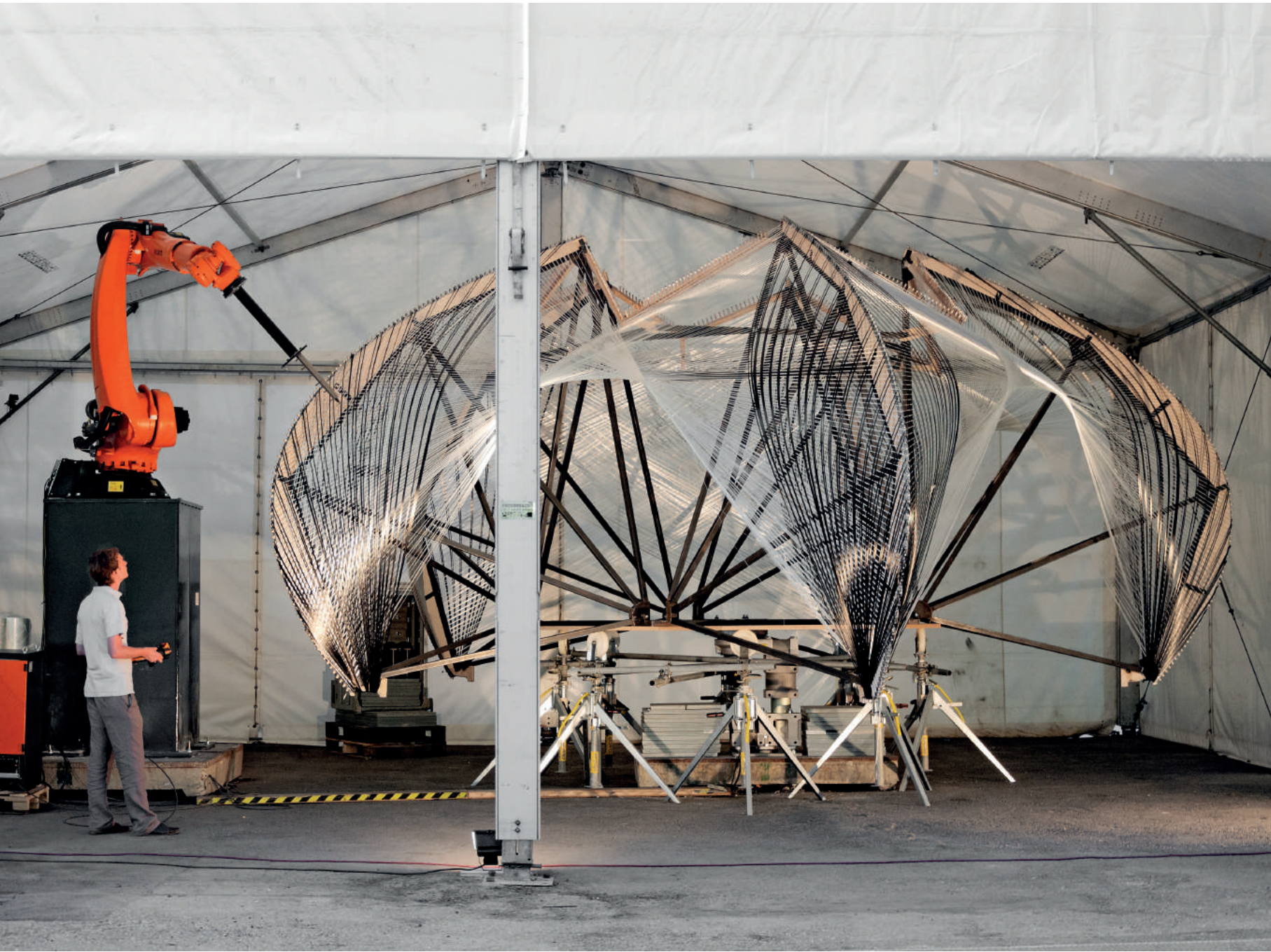
Fig. 1: Institute for Computational Design, Institute of Building Structures & Structural Design, Faculty of Architecture and Urban Planning, University of Stuttgart, ICD/ITKE Research Pavillion, Robotic Carbon and Glass Fibre Winding, Stuttgart, 2012.
