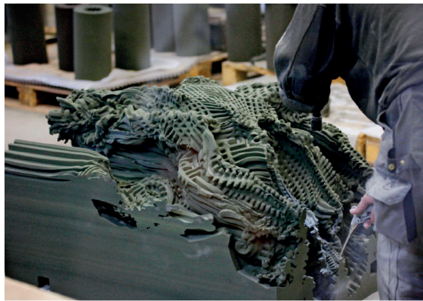
Fig. 4: Sand removal from printed grotto element.
