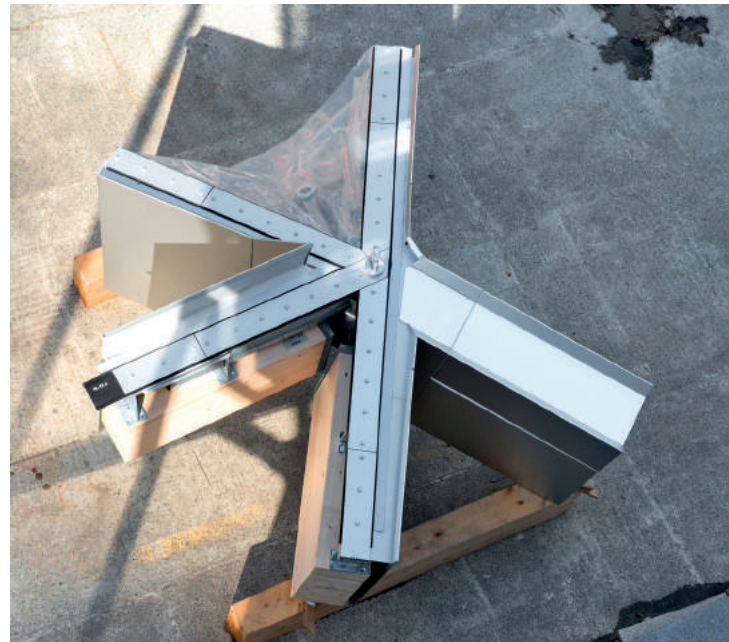
Fig. 4: Photograph showing mock-up of single node (ID 28) with five connecting timber glulam beams. The mock-up shows the ETFE frames, ETFE cushion fabric, timber flashings, and air distribution system integrated into support brackets. Visible also is the deviation of the timber and ETFE frame axes along the diagonal beams. (Photo: Nigel Young / Foster + Partners.)
