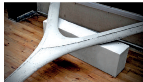
Fig. 9: Y-joint sample cast constructed from three intersecting hyperbolic paraboloidal surfaces and six single-ruled extrusions.
