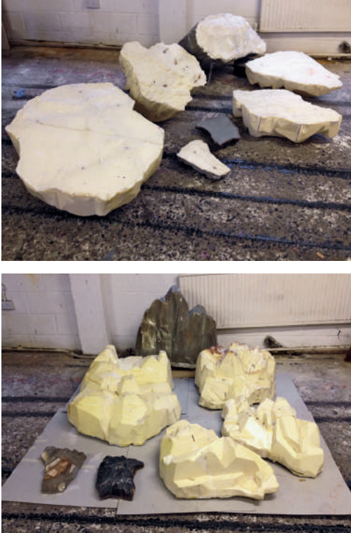
Fig. 9: The full collection of positive replicas. Each combines a SLA top surface and a high-density foam carved underside.
