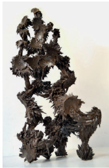
Fig. 6: MAGNETIC ARCHITECTURE Project, developed by Gabriel Bello, Alexandre Dubor, Akhil Kapadia, Angel Lara. FABbots 3.0. IaaC, 2012. Left: Custom-made, digitally controlled magnetic clamp. (Photo: Jordi Portell.) Right: Complex formation of iron and binder matter, built with a magnetic clamp that can be positioned in multiple directions. (Photo: Akhil Kapadia.)
