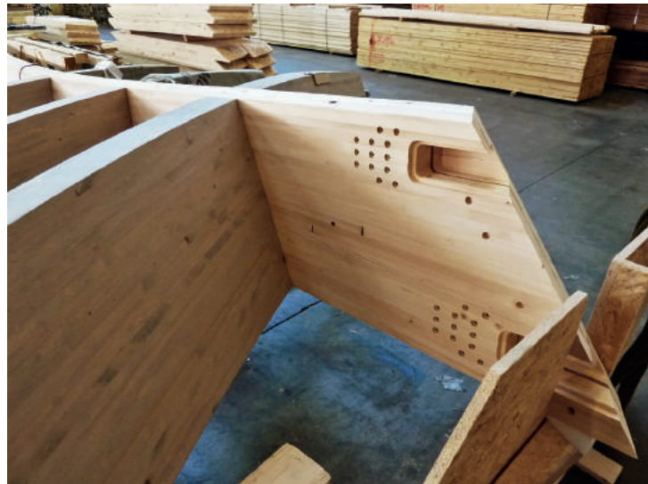
Fig. 12: The single-curved beams feature five-axis contours and a wide variety of different drillings, slots and pockets. (Hess Timber.)
