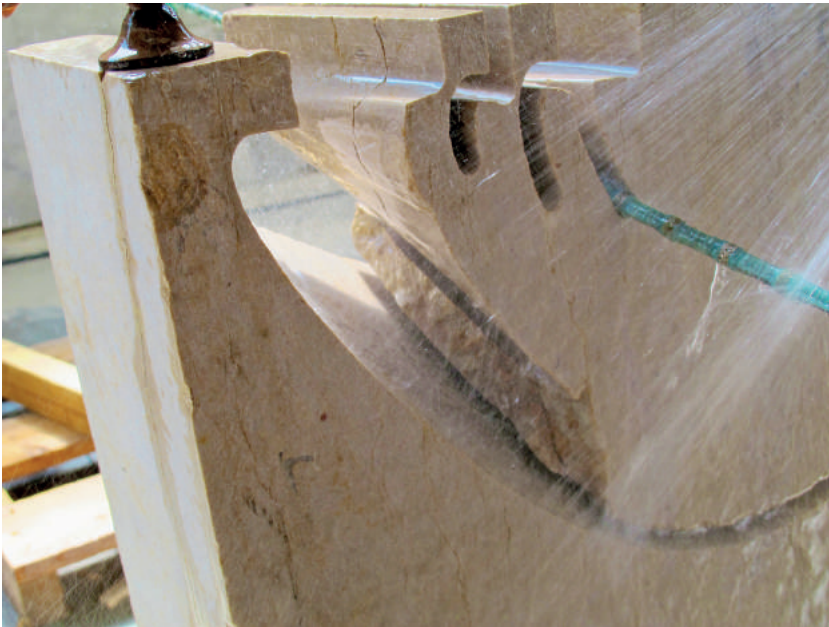
Fig. 5: Application of abrasive wire swing at the quarries in Carrara, Italy.
