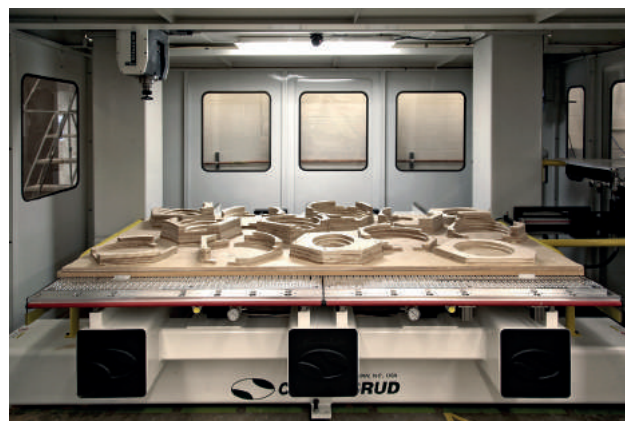
Fig. 7: Roughed aggregated blanks of the desired geometry await the milling operation on the five-axis machine.
