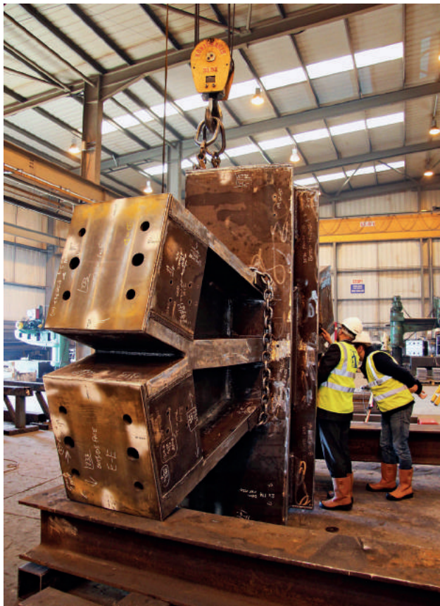
Fig. 6: Node type 7 in fabrication. Node 7 incorporates the thickest plate sizes of the entire Megaframe (180 mm).
