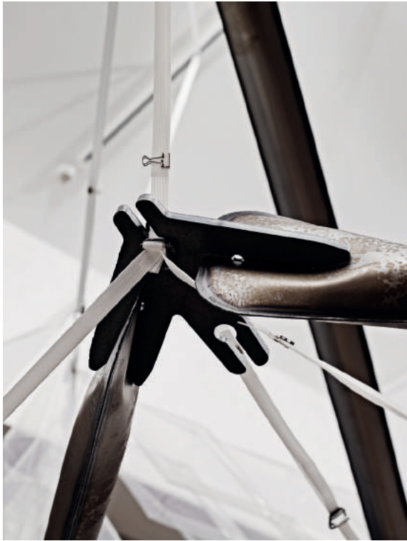
Fig. 7: Persistent Model #2: One aspect of the project investigates a novel form of junction for steel structures that employs metal inflation and resolves the need for conventional means of mechanical fixing. (Photo: Anders Ingvarsten.)
