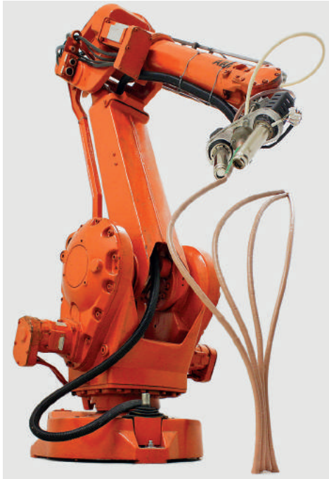
Fig. 7: Surfaces and objects can be formed by combined 3D curves instead of successive 2D layers allowing more control over the fabrication process. (Image by courtesy of Joris Laarman Lab.)
