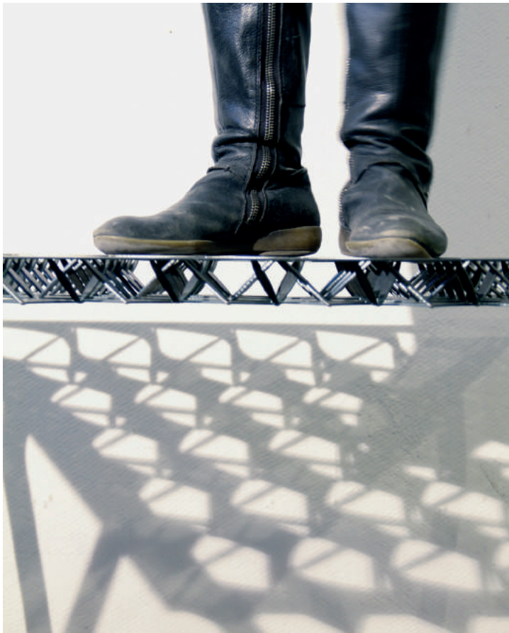
Fig. 5: Prototype in steel exhibiting structural capacity and light transmission. (Photo: D. Skidmore.)
