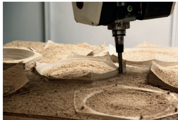
Fig. 8: Swarf milling the voussoir edges.
