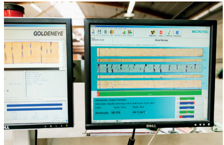
Fig. 5: Photograph showing computer monitoring of machined timber for grade evaluation and visual inspection, including numbers of knots and other defects. Wiehag Factory, Altheim, Austria. (Photo: Nigel Young / Foster + Partners.)
