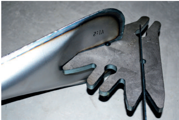
Fig. 9: Avoiding penetrative methods of connection preserves the integrity of the metal cushion, making it possible for discrete phases of inflation to be conducted arbitrarily.
