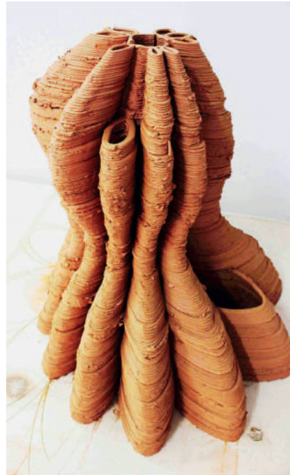
Fig. 2: FABCLAY Project, developed by Nasim Fashami, Saša Jokić. Starski Naya. FABbots 3.0, IaaC, 2012. Printed building component in clay, specifically programmed for continuous material flow. (Photo: Saša Jokić.)
