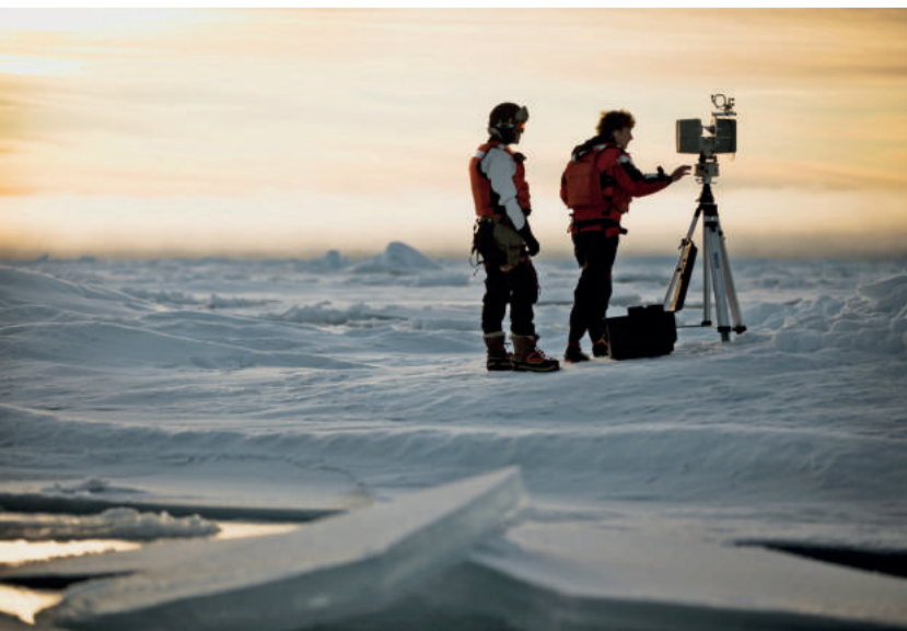
Fig. 3: 3D scanning of the top surface of Arctic ice floes in the Fram Strait, northwest of Svalbard, Norway.
