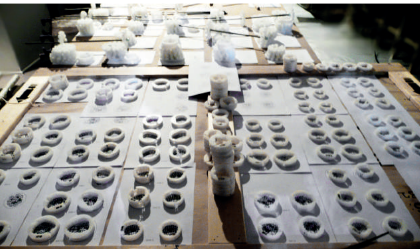
Fig. 19: Star nodes and packing nodes arranged according to installation order.
