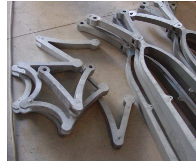
Fig 8.22 Cast aluminium and maple stair in Tudor House, architect Knox Bhavan, 2003
