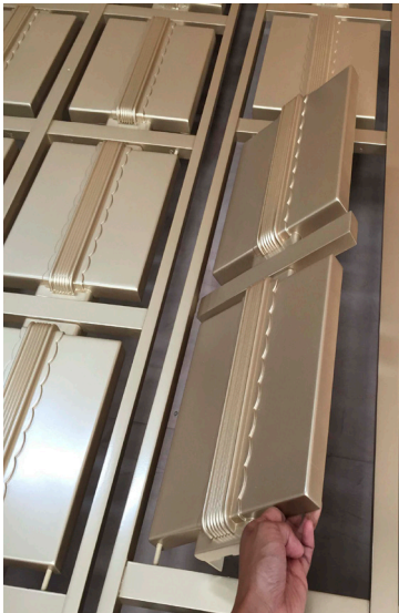
Fig 6.16 Detail of the liquid-metal coated aluminium facade screens
