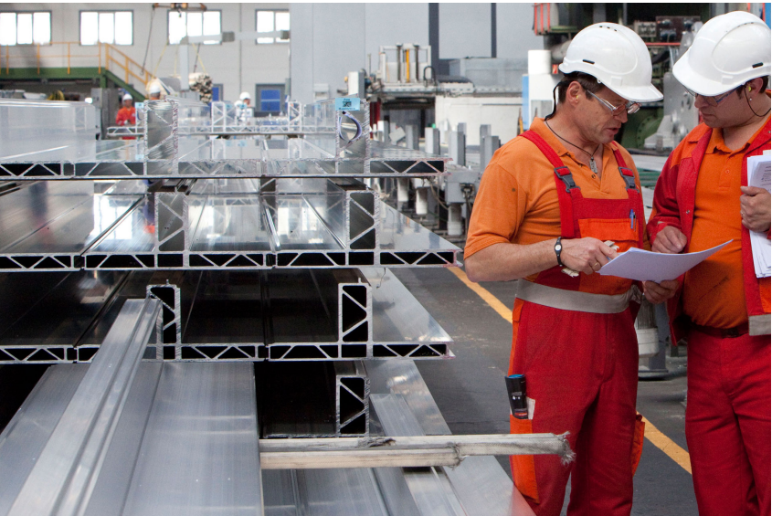
Fig 1.19 Large format aluminium alloy extrusions in Constellium's plant, Singen, Germany
