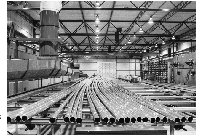
Fig 1.4 Extruded aluminium tubular sections ready for straightening at Sapa, Tibshelf Plant, Derbyshire, England, architect, Foster Associates, 1973
