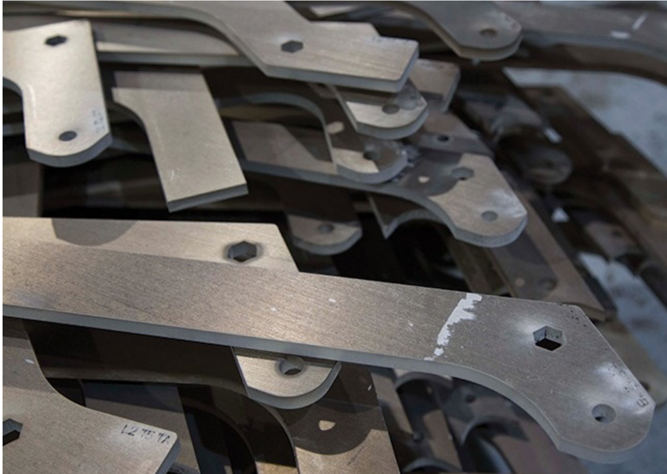
Fig 2.11 The waterjet cut components of the Hive in Stage One's workshop in York, England
