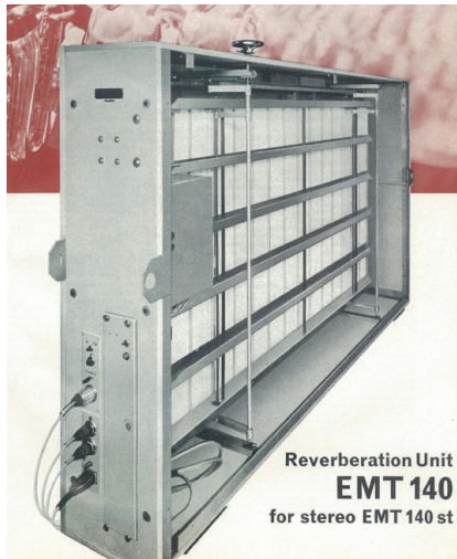
Image 14 (top) Illustration of a plate reverb unit from 1957. A suspended thin steel plate outfitted with pick ups added artificial 'space' to a recording. A secondary damping plate allowed for adjustable reverberation time.
