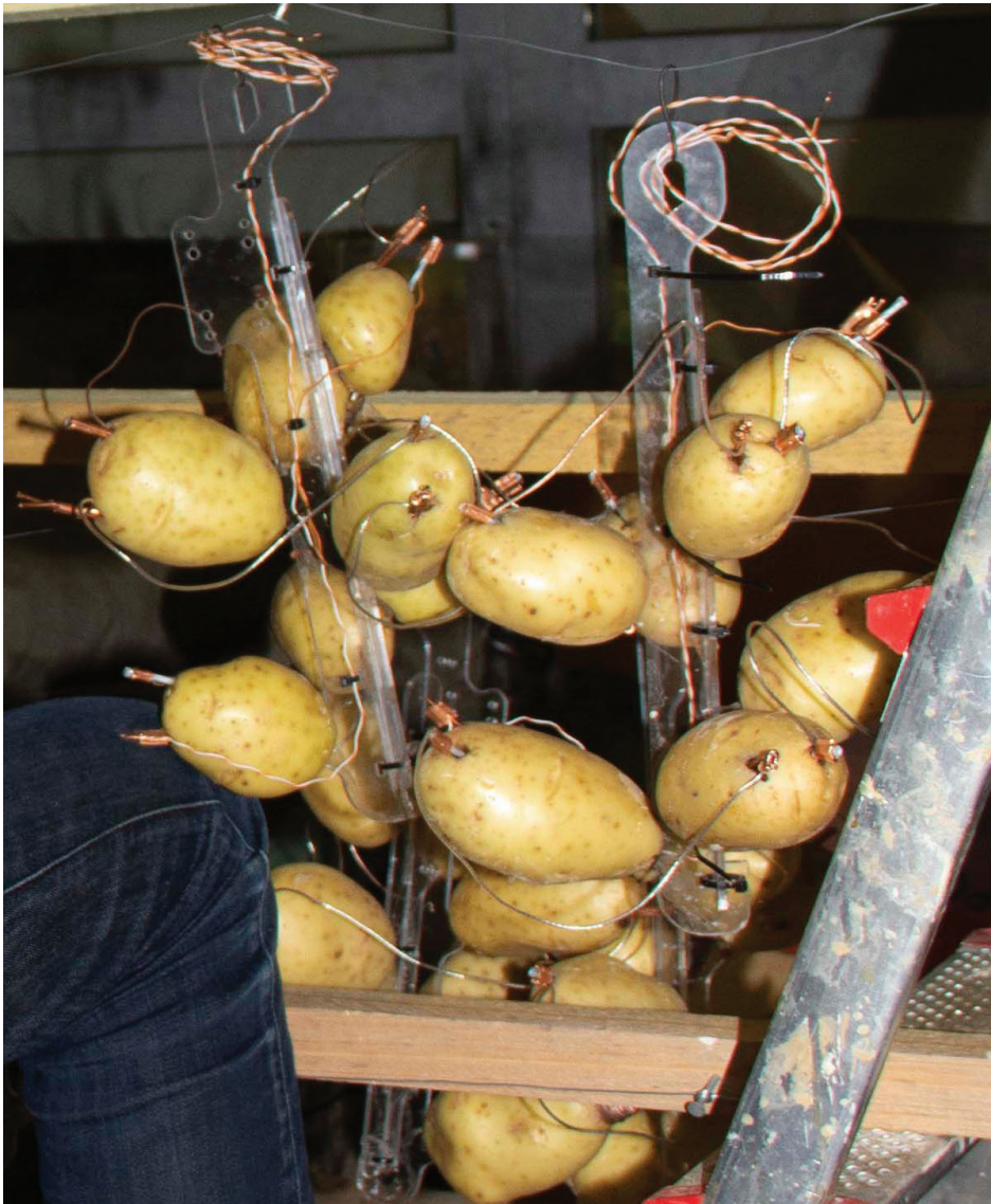
above Potato cells within a pair of potato batteries
